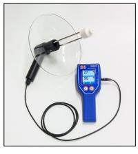
The AR-Loc external directional microphone with a parabolic antenna allows for efficient analysis of discharge activity remotely at distances up to 100 m with the accuracy m. of 1 The sensitivity gain is +20dB.
