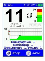
First in this mode, the database of the monitored equipment is created with iNVA software, and all the points for periodic PD measurements are defined. This mode is for routing way of the measurements. The measurement route is generated on PC and is downloaded into the device. The measurements are taken according to the given route; the data is stored in the device memory and is easily transferred into iNVA database. In addition, the routing information
