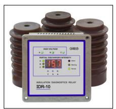
«IDR-10» measuring device is mounted on the front of the switchgear. The three LEDs relay indicate the presence of voltage on the switchgear busbars and its correspondence to the nominal voltage fluctuation range. PD intensity is shown by digital indicator. If PD level exceeds the critical one, then the signal LEDs lit up and the output electromagnetic relay switches on.
